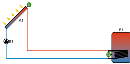
Internal heat exchanger, intelligent pump control
