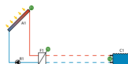
Stand-alone operation of the external heat exchanger, intelligent pump control
